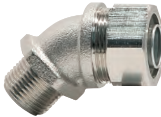
LIQ20E45 (IP66/67/68) External Male Thread 45 degree bend Multi part compression fitting with a nylon seal Available in Nickel Plated Brass (NPB) and 316 Stainless Steel (SS)
