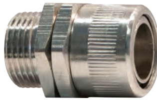
CSFSC - BSW (IP40) Two part brass nickel plated straight fitting with a swivel external male thread. Can be installed into a threaded entry or a knockout and secured by a lock nut.
