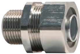
LIQ20T (IP66/67/68) External Male Thread Straight Multi part compression fitting with a nylon seal Available in Nickel Plated Brass (NPB) and 316 Stainless Steel (SS)
