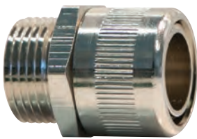
CSFSC - B (IP40) Two part brass nickel plated straight fitting with a fixed external male thread. Can be installed into a knockout and secured by a lock nut.
